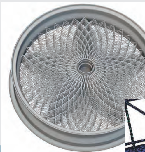
金属積層造形部品解析 (nTopによる複雑構造適用評価) Metal additive manufactured parts analysis (Complex structure application evaluation via nTop)
