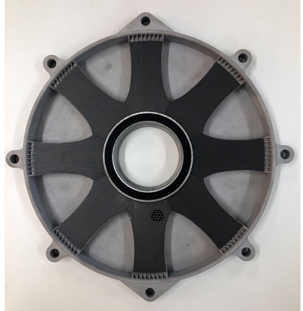
Development Product (CFRP+ Aluminium Additive Manufacturing Product)
