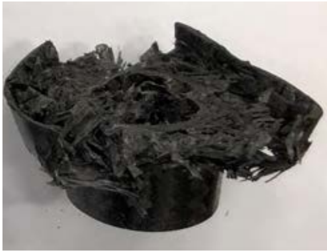
Compression test results (CFRP)(with knife edge)
