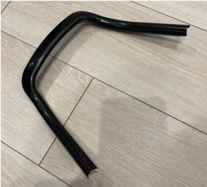
Prepreg autoclave molding (CFRP) Molding time (from material cutting to demolding): approx. 300 min.
