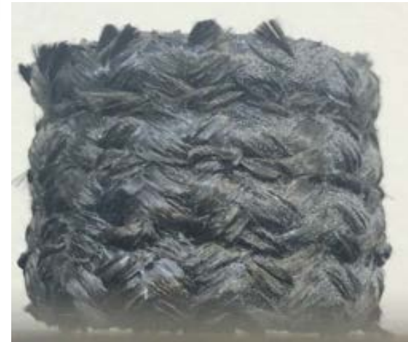
Compression test results (CFRTP)(without knife edge)
