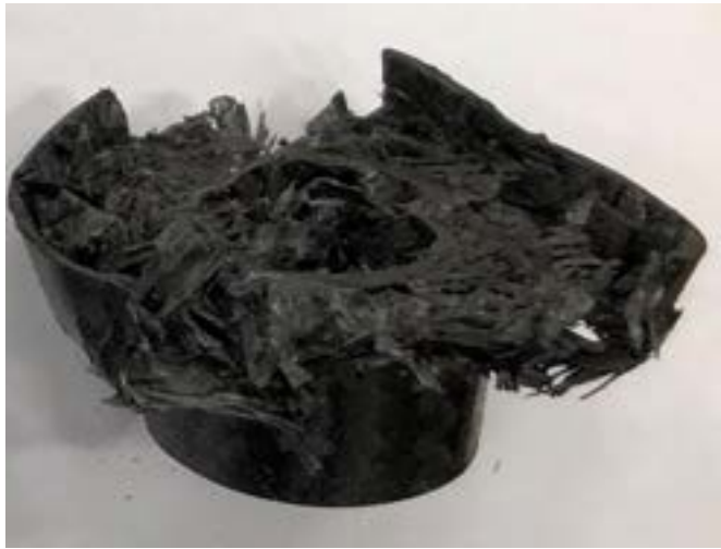
Compression test results (CFRP)(with knife edge)
