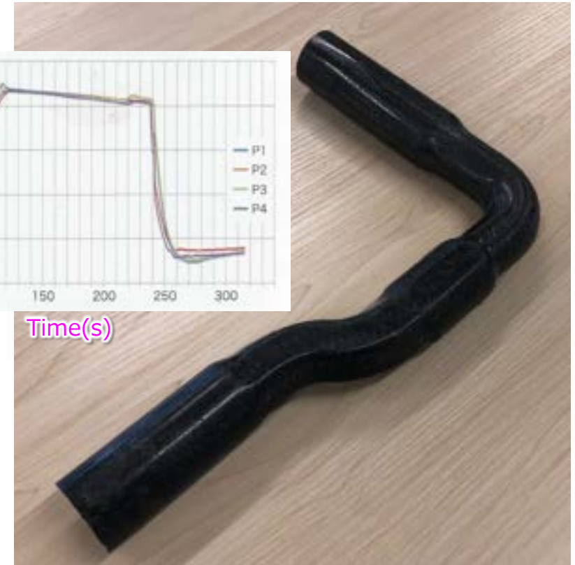
Commingled braids internal pressure molding (CFRTP) Molding time (from material cutting to demolding): Approx. 15 min.
